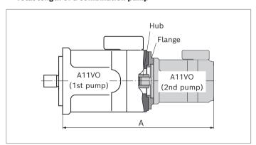
When using the Z-shaft (splined shaft DIN 5480) for the mounted pump (2nd pump)
