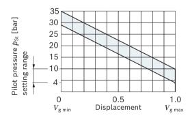
Pilot pressure increase  $V_{\rm g \ max}$  to  $V_{\rm g \ min}$ :  $\Delta p$  = 25 bar
