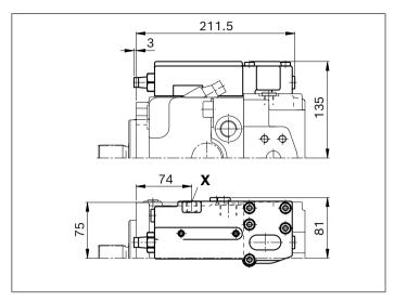
▼ LE2S - Power controller, electrical override, load-sensing (negative control)
