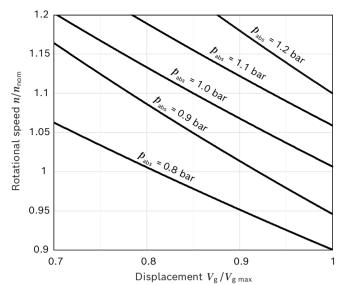
Permissible rotational speed depending on inlet pressure  $p_{\rm absolute}$  and displacement volume  $V_{\rm g}/V_{\rm g \ max}$ . Observe the maximum rotational speed  $n_{\rm max}$
