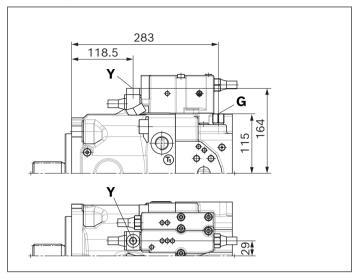
▼ LR3DS - Power controller, high-pressure related override, pressure cut-off, load-sensing
