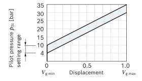
Pilot pressure increase  $V_{\rm g \ min}$  to  $V_{\rm g \ max}$ :  $\Delta p$  = 25 bar
