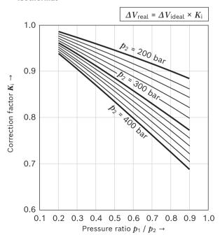
**2.** For an **adiabatic state change**, i.e. a quick change of the gas cushion accompanied by a temperature change of the nitrogen, the following applies:
