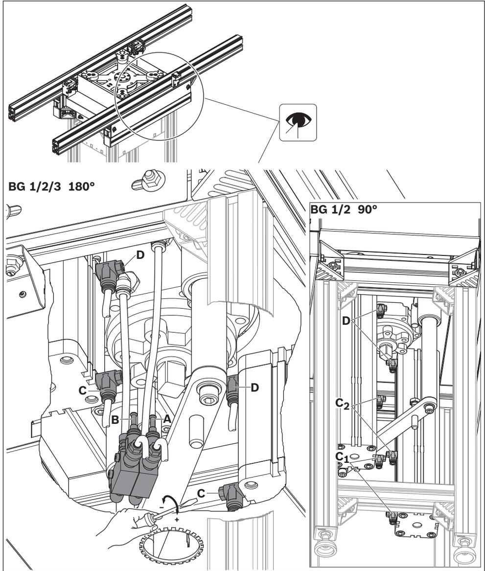
**Fig. 22: Adjust stroke, lift and rotate speed (example shown here size 2)**
