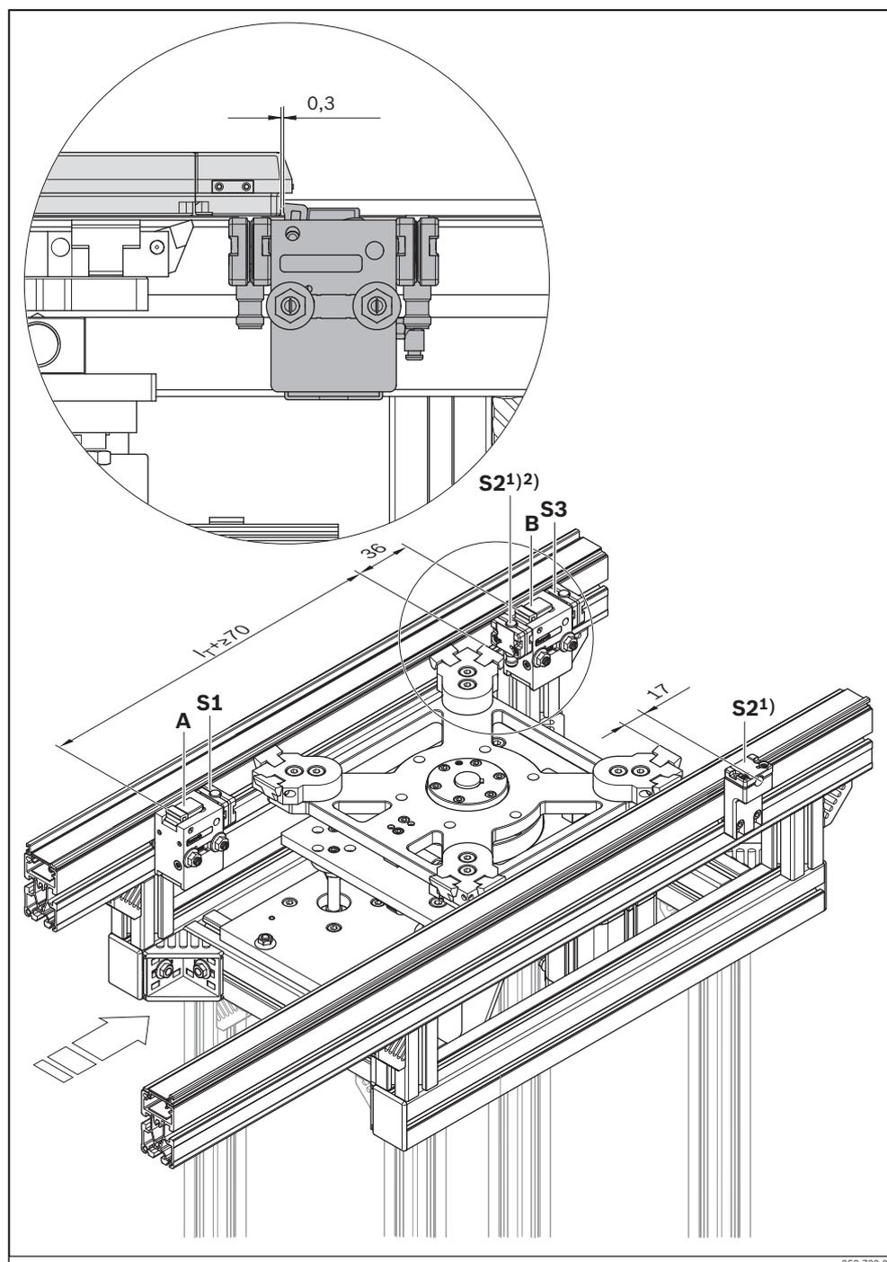
**Fig. 12: Install separator stop and proximity switches (example shown here size 2 180°)**
