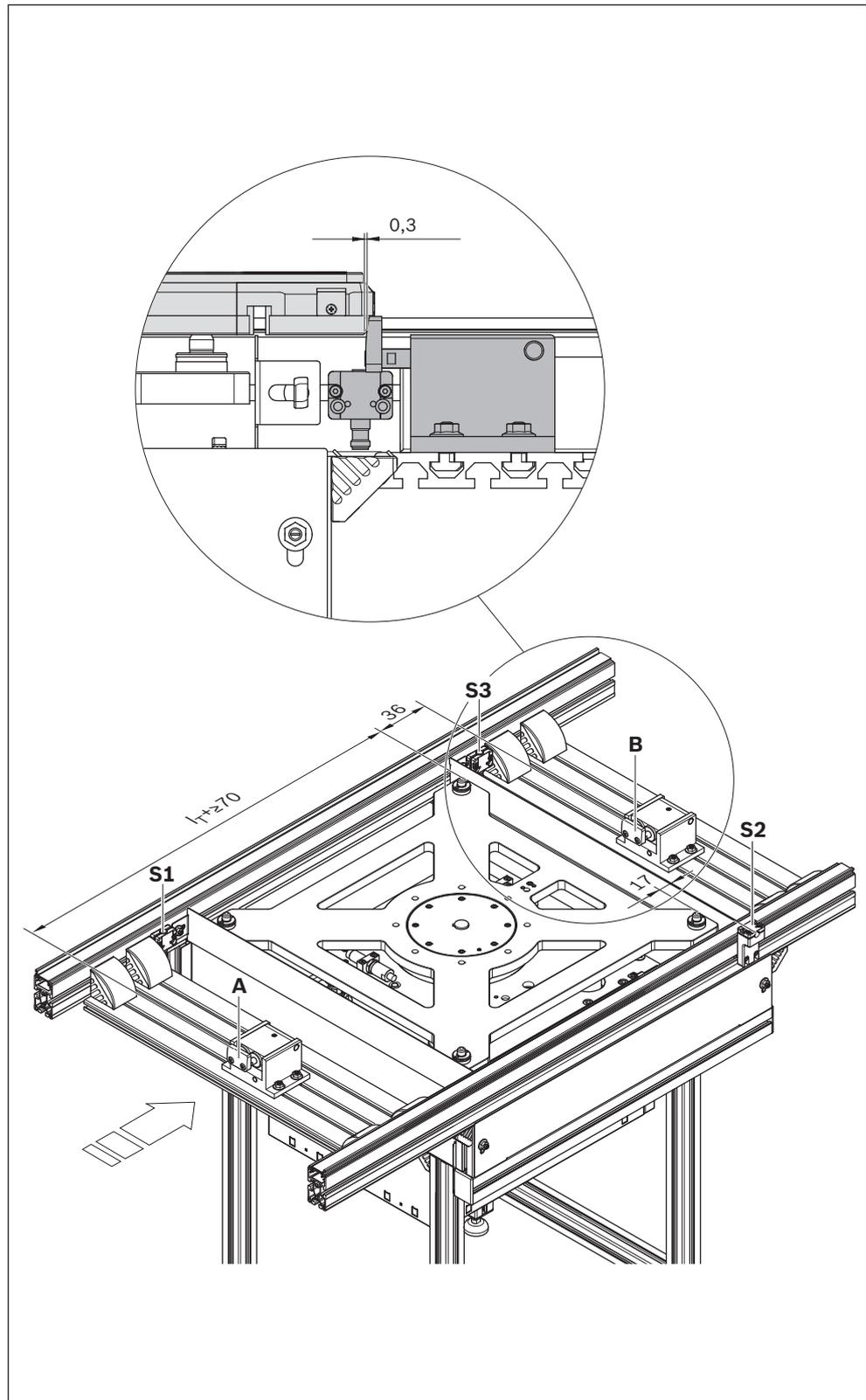
Fig. 13: Install separator stop and proximity switches (example shown here size 3 180°)
