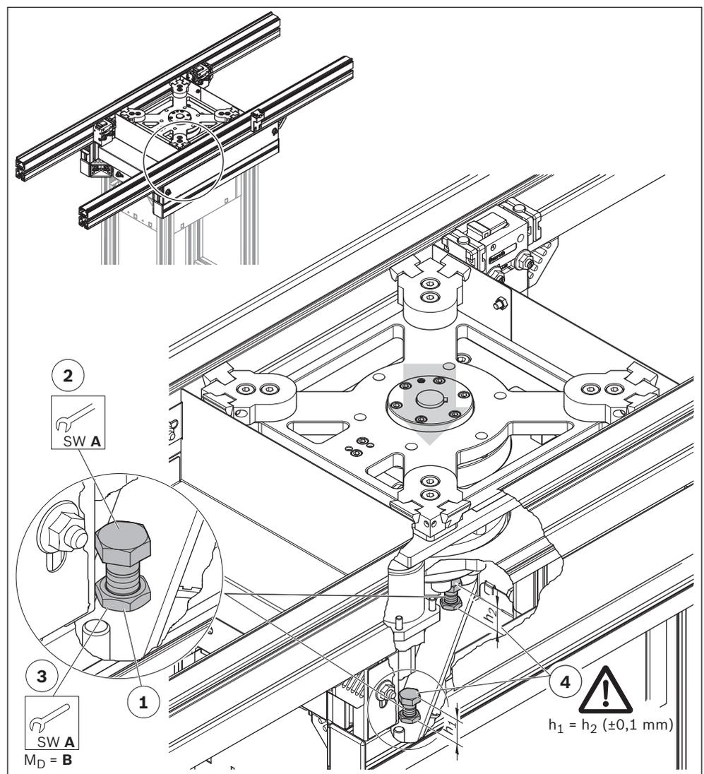
Fig. 23: Set the stroke over the conveyor level (example shown here size 2 180°)
