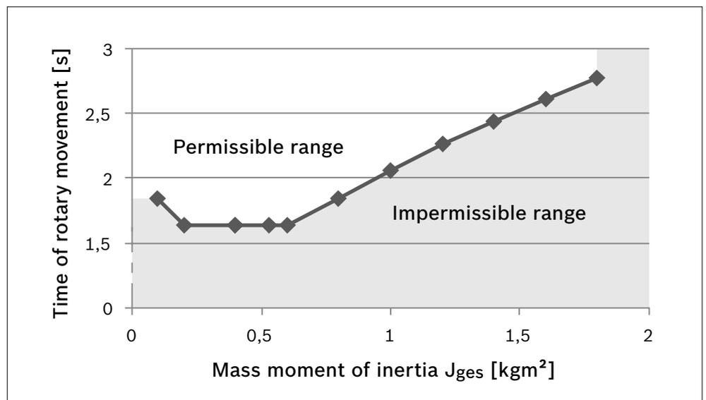
Fig. 30: Diagram mass moment of inertia size 1
