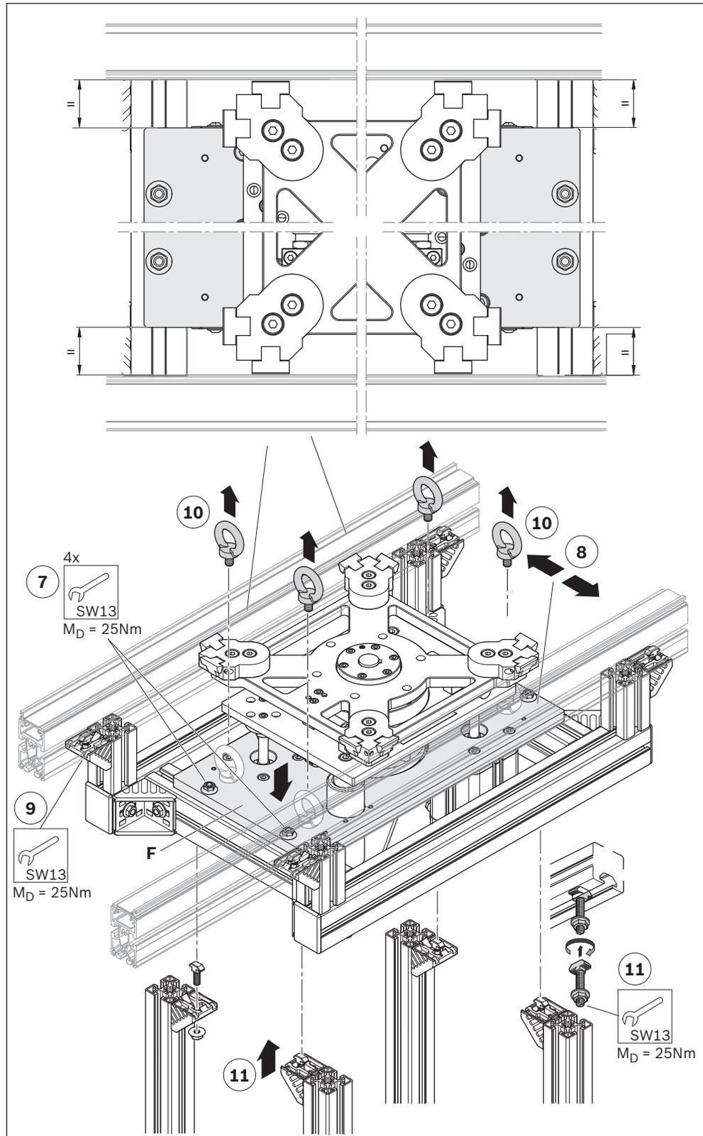
Fig. 9: Adjust lift rotate unit HD 2/H size 2 and 3 in section ST 2 (example shown here size 2 180°)
