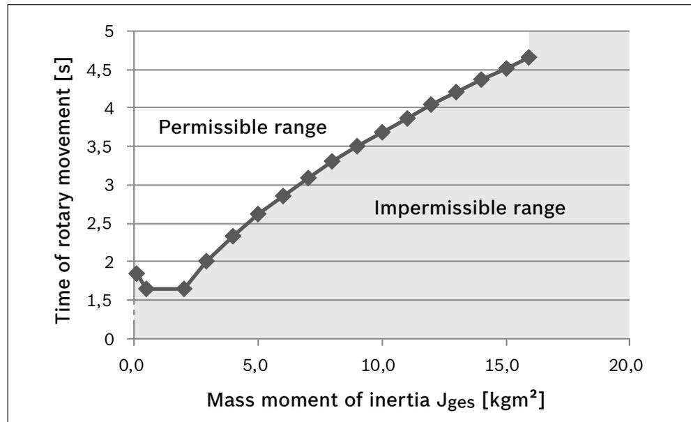
Fig. 31: Diagram mass moment of inertia size 2
