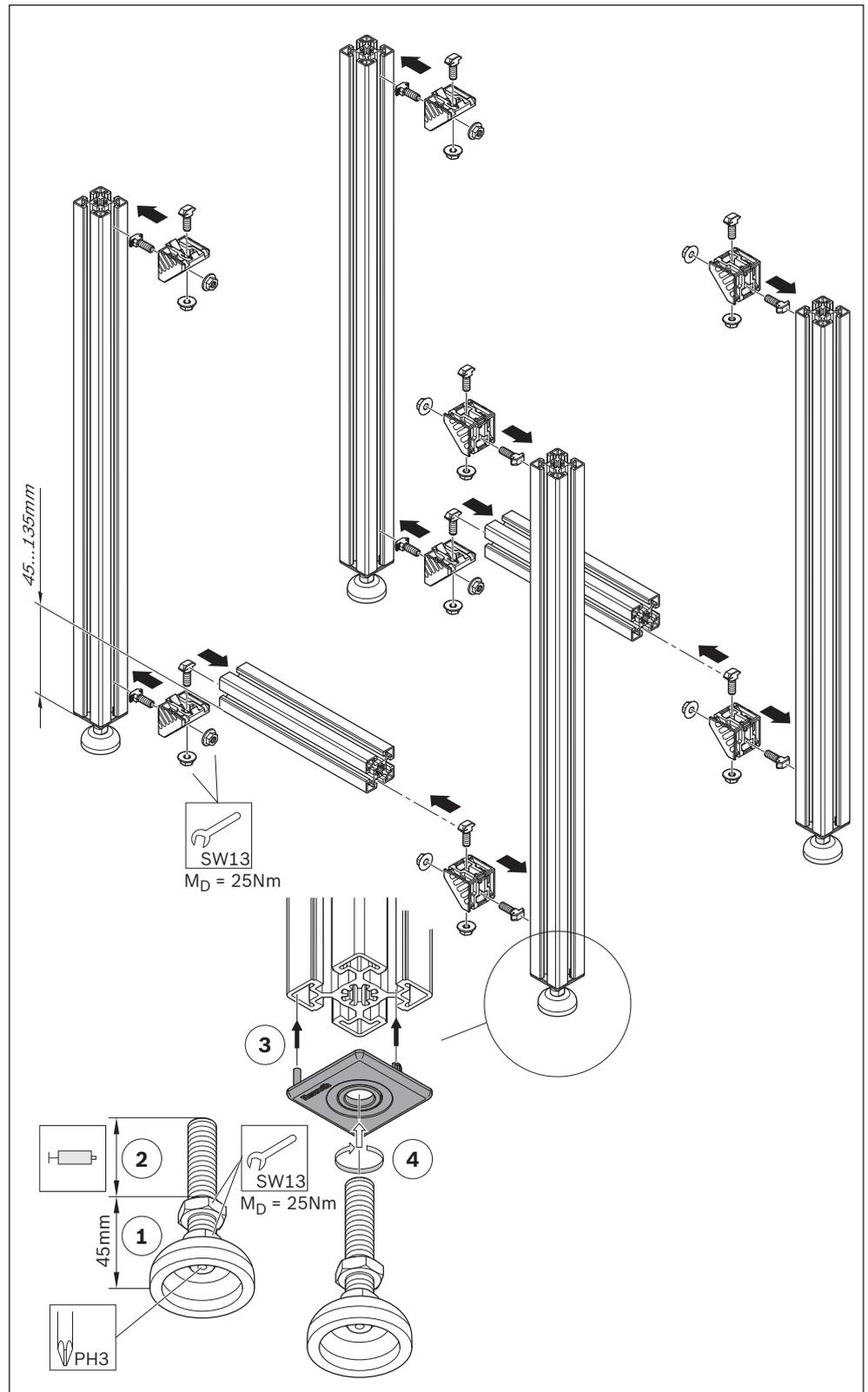
**Fig. 10: Install the additional supports**
