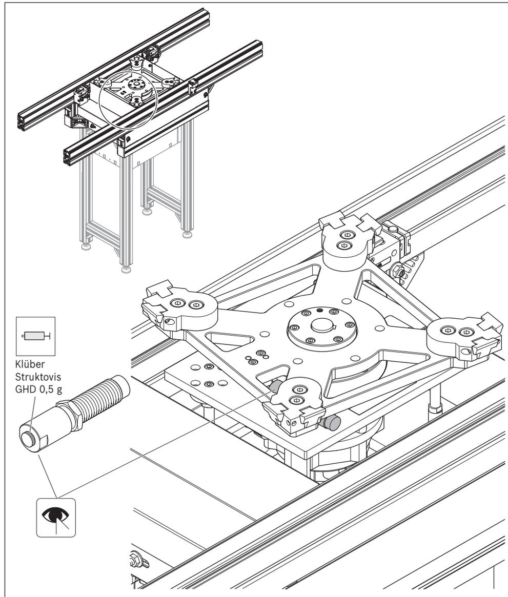
Fig. 27: Lubricate the load adapter damper
