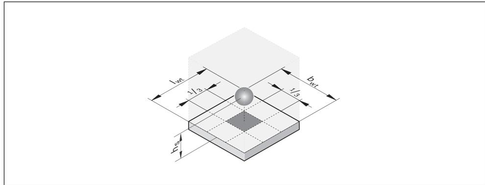
Fig. 25: Center of gravity on the workpiece carrier
