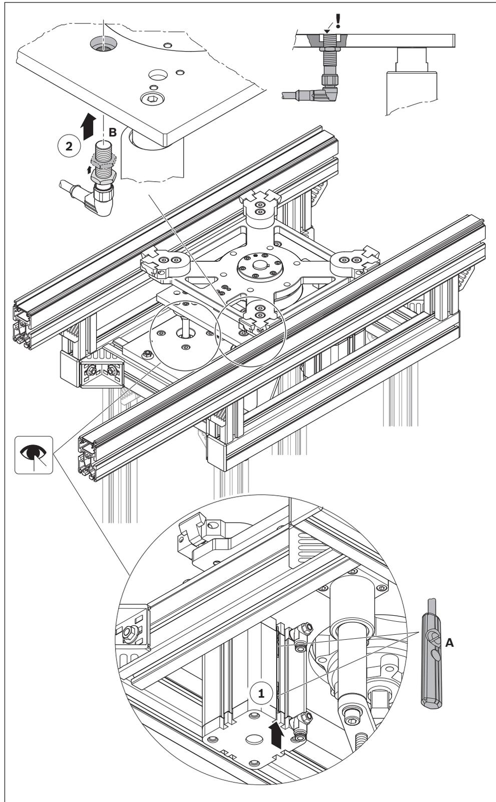
**Fig. 11: Install position query for vertical lift and horizontal rotation (example shown here size 2 180°)**
