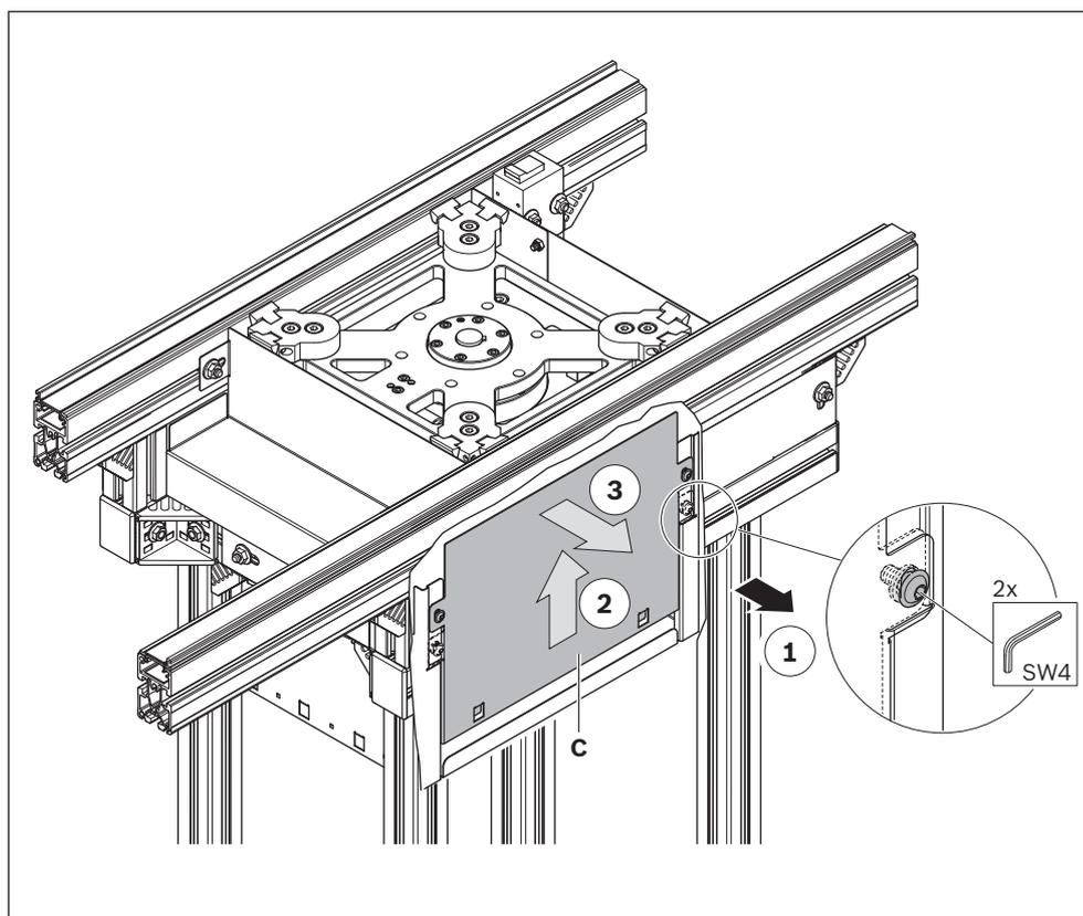
Fig. 18: Open inspection openings
