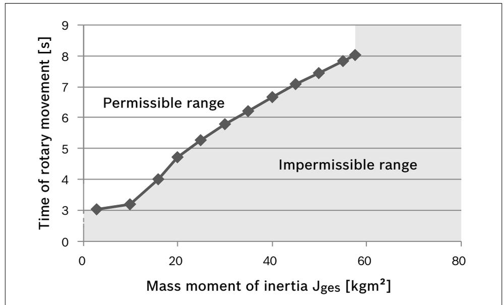
Fig. 32: Diagram mass moment of inertia size 3
