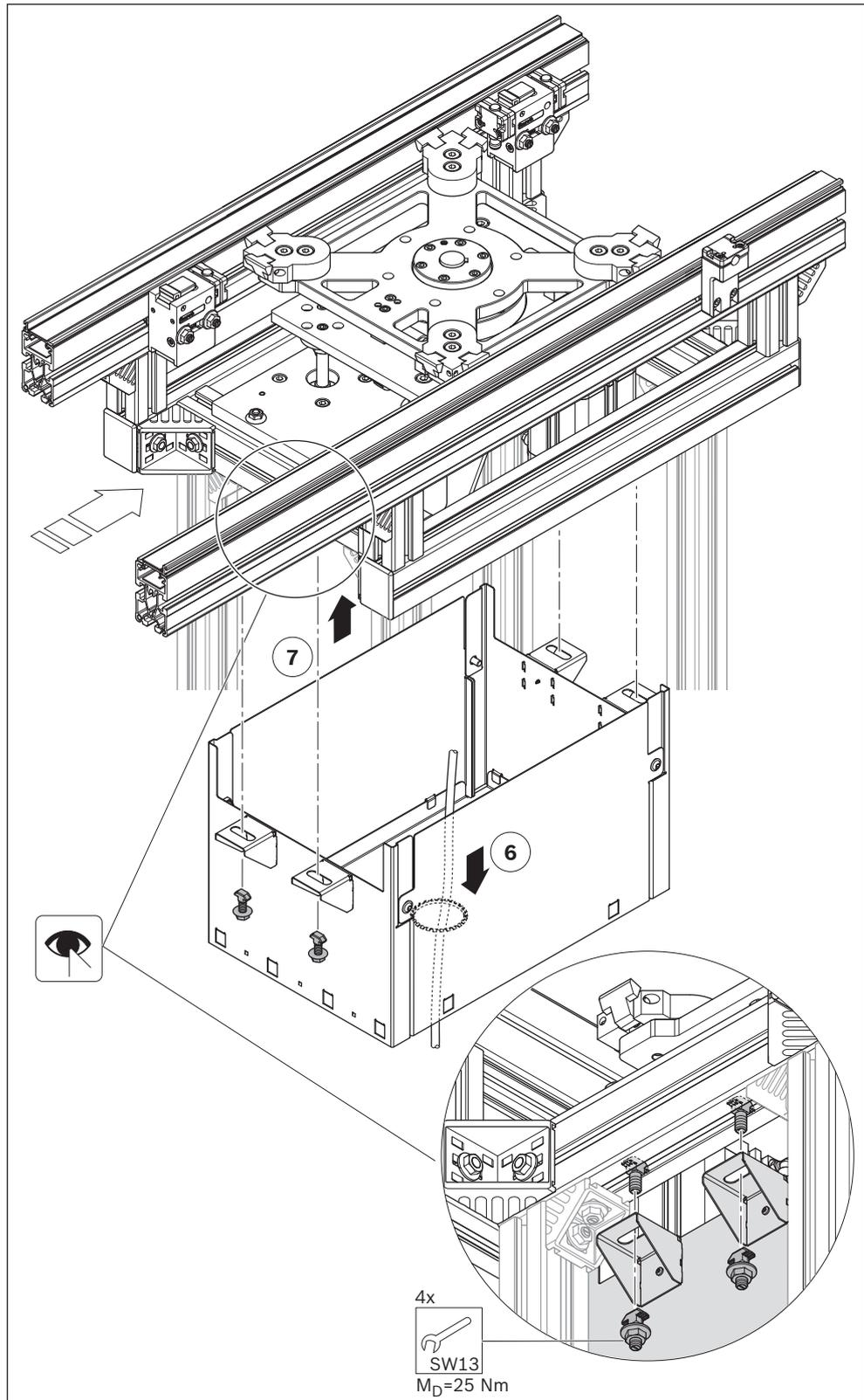
Fig. 15: Install protective case (example shown here size 2 180°)
