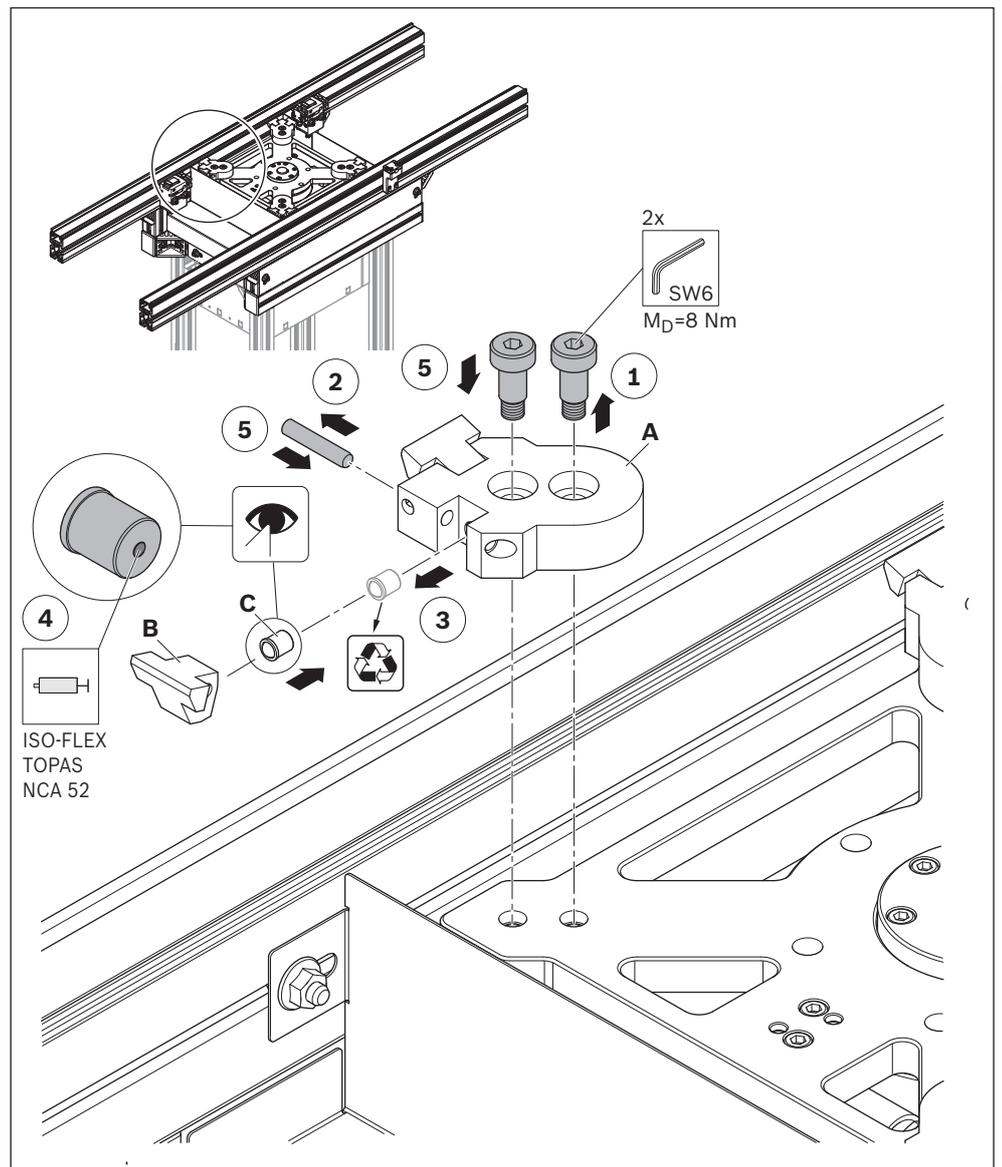
Fig. 28: Exchange the pressure point of the fingers in the rotary table (only sizes 1 and 2).
