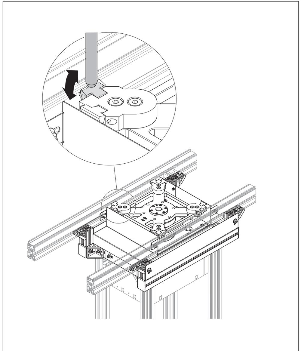
**Fig. 26: Check the spring action of the pressure point**
